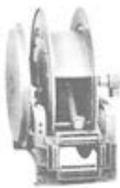
Series 700/800/900. Spring rewind reel that handles to 150 feet of \frac{1}{2} " hose, 110 feet of \frac{3}{4} " hose, 120 feet of 1" hose, and up to 90 feet of 1\frac{1}{2} " hose. The 900 series has pressures up to 600 psi. The 700/800 series has pressures up to 1000 psi.
