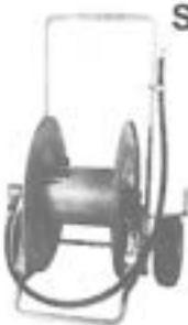
AT 1200. Portable hose reel that handles up to 375 feet of \frac{1}{2} " I.D. hose and up to 900 feet of 1" I.D. hose. Operates at pressures up to 1000 psi.
