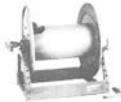
Series 3000/3500. Manual rewind reels that handle \frac{1}{4} ", 1", and 1\frac{1}{2} " hose. Handles pressures to 1000 psi. Reels are equipped with a spring-actuated pin lock.
