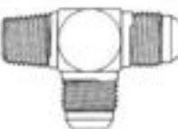
External pipe/37° flare Part no. 2028 (Dash size) (Ref. SAE 070424)
