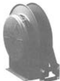
Series N500. Spring rewind reel with J-spring that comes in a narrow frame. Handles up to 80 feet of \frac{1}{4} " hose and 95 feet of \frac{3}{8} " hose. Pressures to 10,000 psi.
