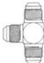
37° flare/37° flare Part no. 20333(Dash size) (Ref. SAE 070401)
