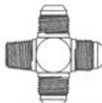
External pipe/37° flare Part no. 202003(Dash size)
